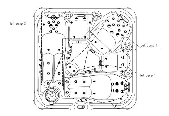
Notes:Due to manufacturing tolerances, there could be some minor differences between the actual spa and the drawing above. If site planning is critical to such tolerances, be sure to measure your actual spa. All specifications are subject to change without notice. Some components may be optional on your spa
